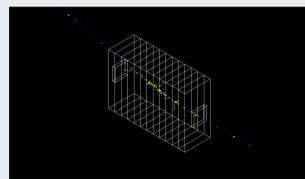
Figure 9: Experiment run with 12 inches of lead. The particle's path is noticeably diverted and a large number of particles are produced due to interaction between the muon and lead.
