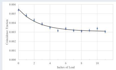
Figure 6: Coincidence Fraction Coincidence fraction is found by dividing the number of coincidences in 24 hours by the total number of counts seen by just the top detector. Equation (2) was used to produce the black curve, and  $C_{hi}$  and  $C_\mu$  were calculated relative to the coincidence fraction values.
