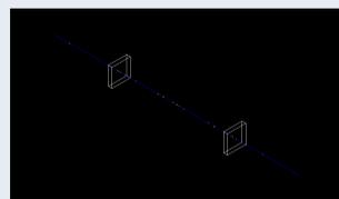
Figure 8: Experiment run with 0 inches of lead. A muon runs straight through the detector with no discernible changes.
