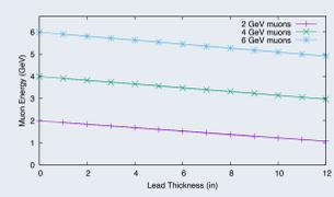
Figure 11: Effect of lead thickness on  $\mu^+$  energy loss. Average value of energy loss from different thicknesses of lead and muon energies of 2, 4, and 6 GeV.
