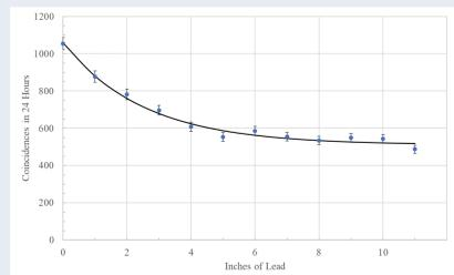
Figure 5: Coincidences in 24 Hours as a Function of Lead Thickness The amount of coincidences observed decreases as the amount of lead between the detectors increases. Equation (2) was used to generate the black curve.
