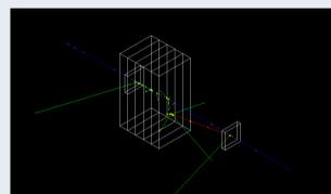
Figure 10: Experiment run with 8 inches of lead. The course of the muon is slightly diverted by the lead, as well as many electrons and gamma rays being produced through the particle's interaction with lead.
